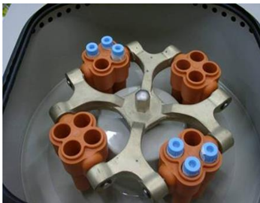
Figure 3. The tubes are centrifuged for ten minutes at 800 rpm, which separates the blood into 3 layers: platelet-poor plasma, platelet-rich plasma, and red blood cells.
